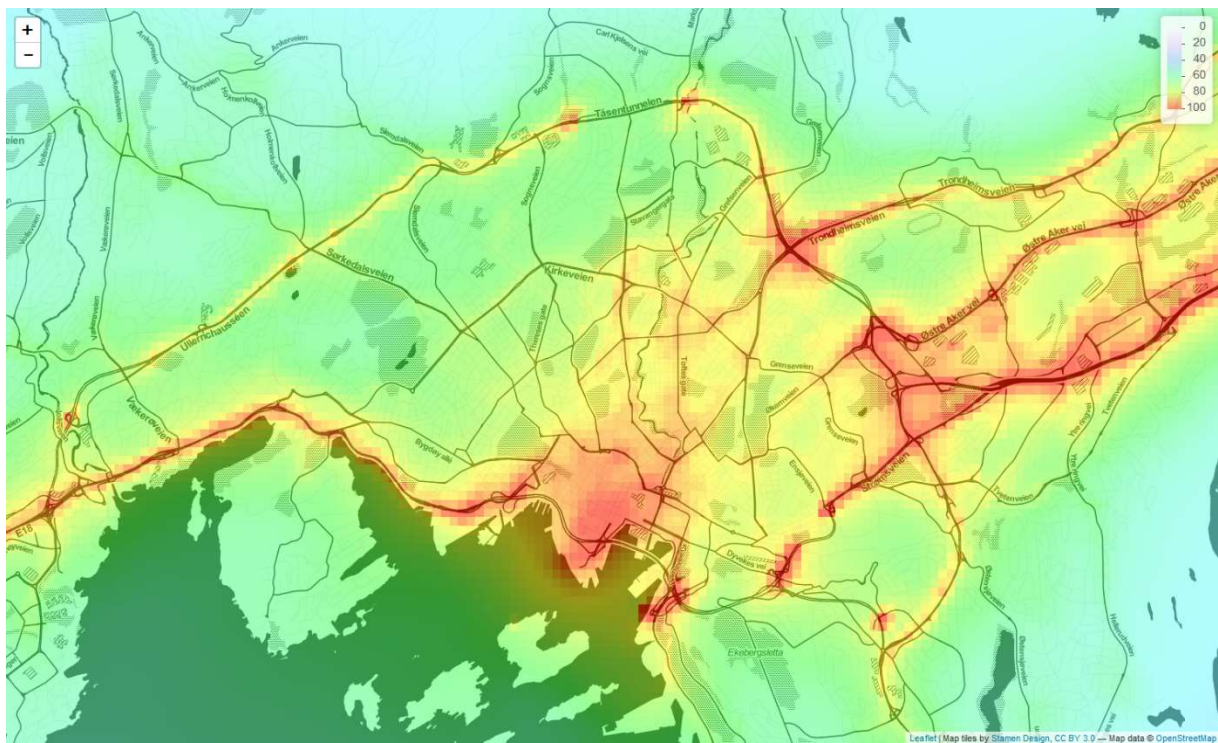
Figure 9-2 Example of a data fusion-based surface concentration field of NO 2 for Oslo, Norway, at 100 m spatial resolution
