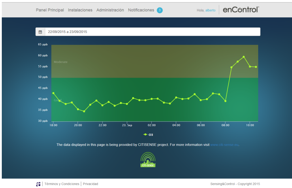
Figure 10-8: Ozone (O 3 ) raw data aggregated (avg) on 30 minute interval with AQI on background.
